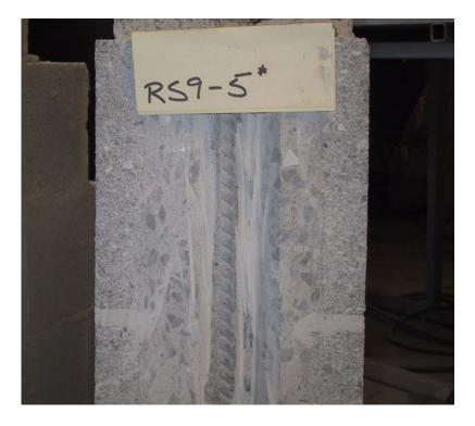
Figure 7. Wall cross-section with Oztec Rebar Shaker consolidation
