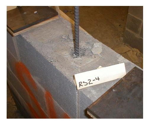
Figure 3. Typical small cone of grout that failed during testing of #4 bars
