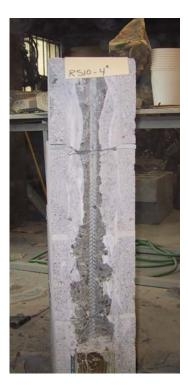
Figure 8. Wall cross-section with Oztec Rebar Shaker consolidation
