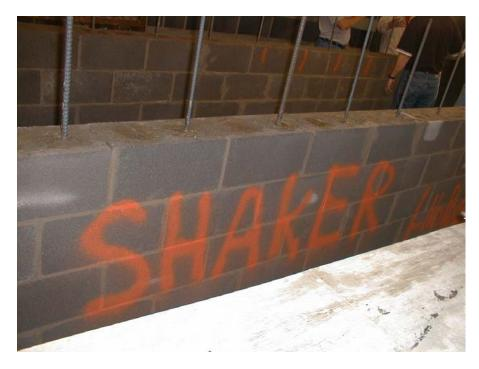
Figure 1. Completed wall prior to testing
