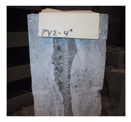
Figure 5. Wall cross-section with pencil vibrator consolidation
