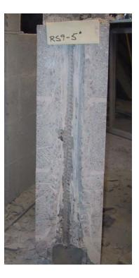
Figure 6. Wall cross-section with Oztec Rebar Shaker consolidation
