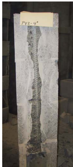
Figure 4. Wall cross-section with pencil vibrator consolidation
